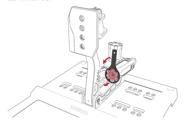
Gently press the pedal to push out the gaskets and elastomers. Do not apply excessive force. 轻压踏板以推出垫圈和胶块。请勿过度用力。
