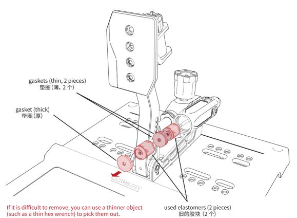
Apply lubricating grease evenly on the cylinder shaft. 在缸轴上均匀涂抹润滑脂。
