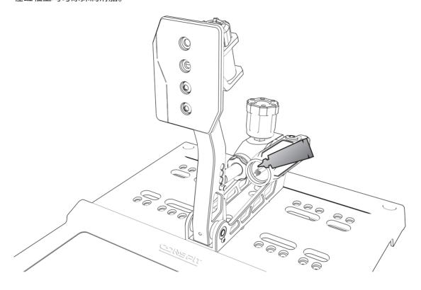
Replace the new elastomers and put the gaskets and elastomers back in their original order. Note: Please replace both elastomers at the same time! 更换新的胶块,并将垫圈和胶块按原顺序放入。注意:请同时更换两个胶块!
