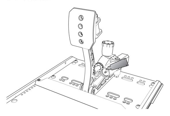
Replace the new elastomers and put the gaskets and elastomers back in their original order. Note: Please replace both elastomers at the same time! 更换新的胶块,并将垫圈和胶块按原顺序放入。注意:请同时更换两个胶块!
