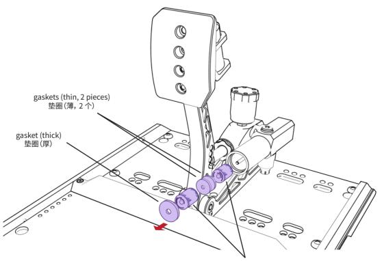
If it is difficult to remove, you can use a thinner object (such as a thin hex wrench) to pick them out. 若难以取出, 可使用较细的物品 (如较细的内六角扳手) 挑出。 used elastomers (2 pieces) 旧的胶块(2 个) Apply lubricating grease evenly on the cylinder shaft. 在缸轴上均匀涂抹润滑脂。
