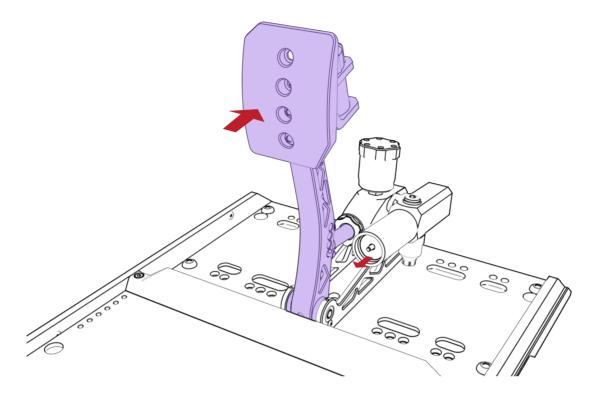
Remove the gaskets and used elastomers. 取出垫圈胶块。
