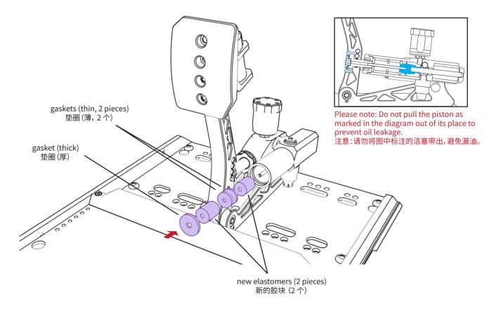
Push the gaskets and elastomers into the cylinder. 将垫圈和胶块推入胶缸。
